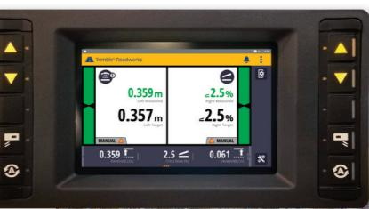
The Trimble Roadworks 2D display features tactile keypads for use in the field
