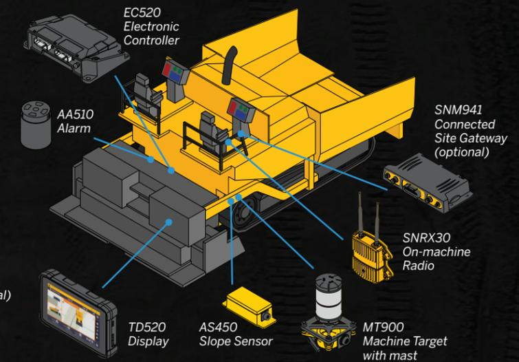
The Trimble Roadworks 2D system can reference off a surface, cross-slope or stringline, making it an excellent, lower cost option for roads that have been graded or milled using Trimble 3D paving control systems.
