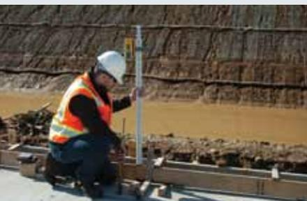
The Spectra Precision® DR400 DigiRod™ eliminates the need for grade rods when checking grades with a rotating laser. The all-in-one combination of a laser receiver with digital readout, laser distance meter, and built-in tilt sensor provide the information required to take rod-less, accurate grade readings, even at tilt angles up to 30 degrees.
