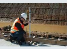
The Spectra Precision<sup>®</sup> DR400 DigiRod<sup>™</sup> eliminates the need for grade rods when checking grades with a rotating laser. The all-in-one combination of a laser receiver with digital readout, laser distance meter, and built-in tilt sensor provide the information required to take rod-less, accurate grade readings, even at tilt angles up to 30 degrees.
